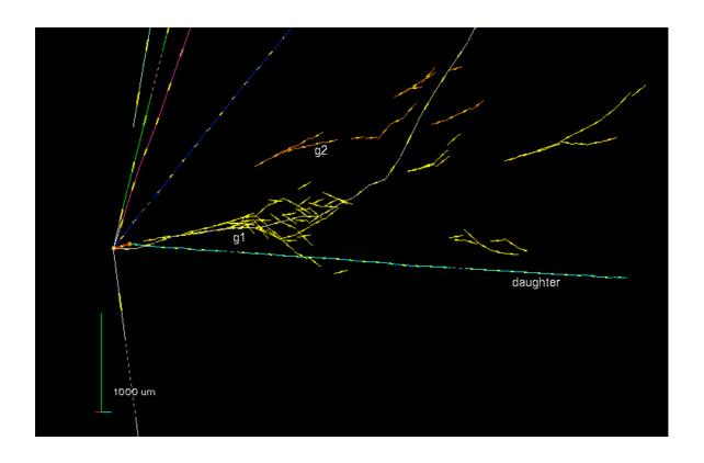
Computer reconstruction of the tau candidate event detected in the OPERA experiment. The light blue track is the one likely induced by the decay of a taulepton produced by a tau-neutrino.
